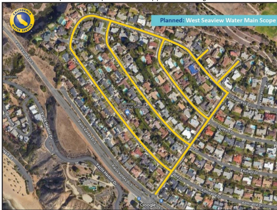
Exhibit 7: Water mains planned to be replaced with flexible pipes in Seaview neighborhood
